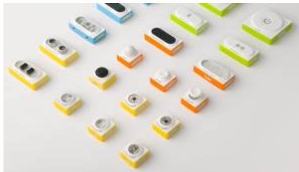
Makeblock Neuron is a programmable electronic building block platform for STEAM education. It contains dozens of different electronic modules such as LED panels, cameras, sensors, ultrasonic, and motors. Through simple combinations, various creative inventions can be created. With the easy-to-use flow-based programming software, the neuron can be “active” without complex code programming to bring concepts and ideas to life.
