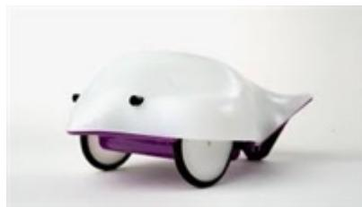
Finch is designed to support an engaging introduction to programming. With support for a dozen programming languages, it allows children to write interactive programs using the robots sensors and motors.
