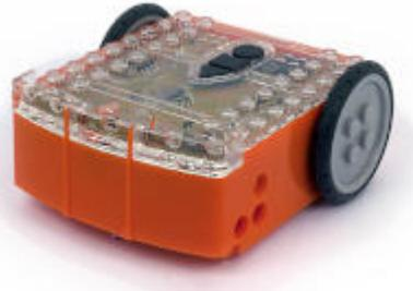
An Australian based robot which is LEGO compatible, the Edison can be converted into a myriad types of machines with the EdCreate extension pages, LEGO blocks, or whatever you might have lying around! Edison can be coded via its own block-based coding language - EdBlocks, or via barcodes, and can be driven with any infra-red remote control unit.
