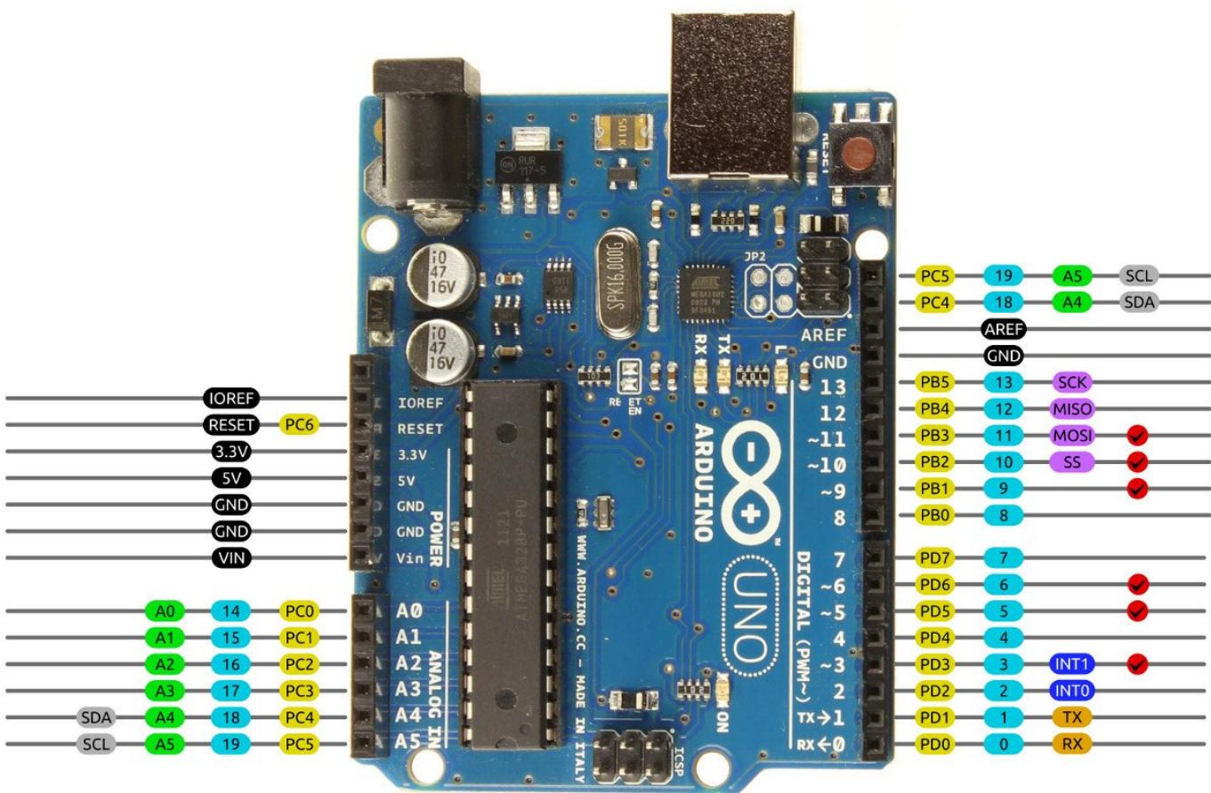
AVR DIGITAL ANALOG POWER SERIAL SPI I2C PWM INTERRUPT
